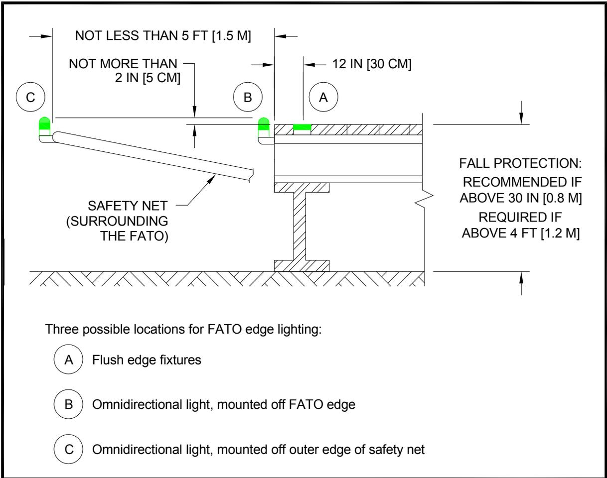
**Figure 3–23. Elevated FATO – Perimeter Lighting: Transport**
