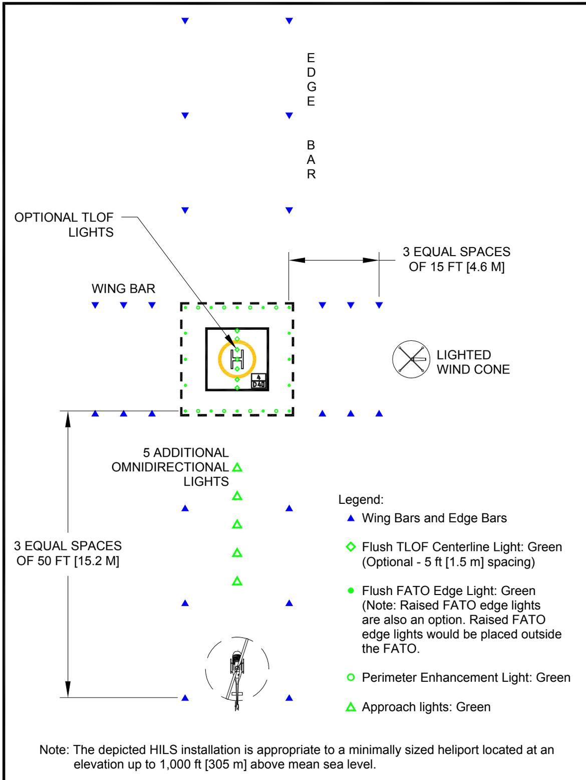
**Figure 6-2. Heliport Instrument Lighting System (HILS): Non-precision**
