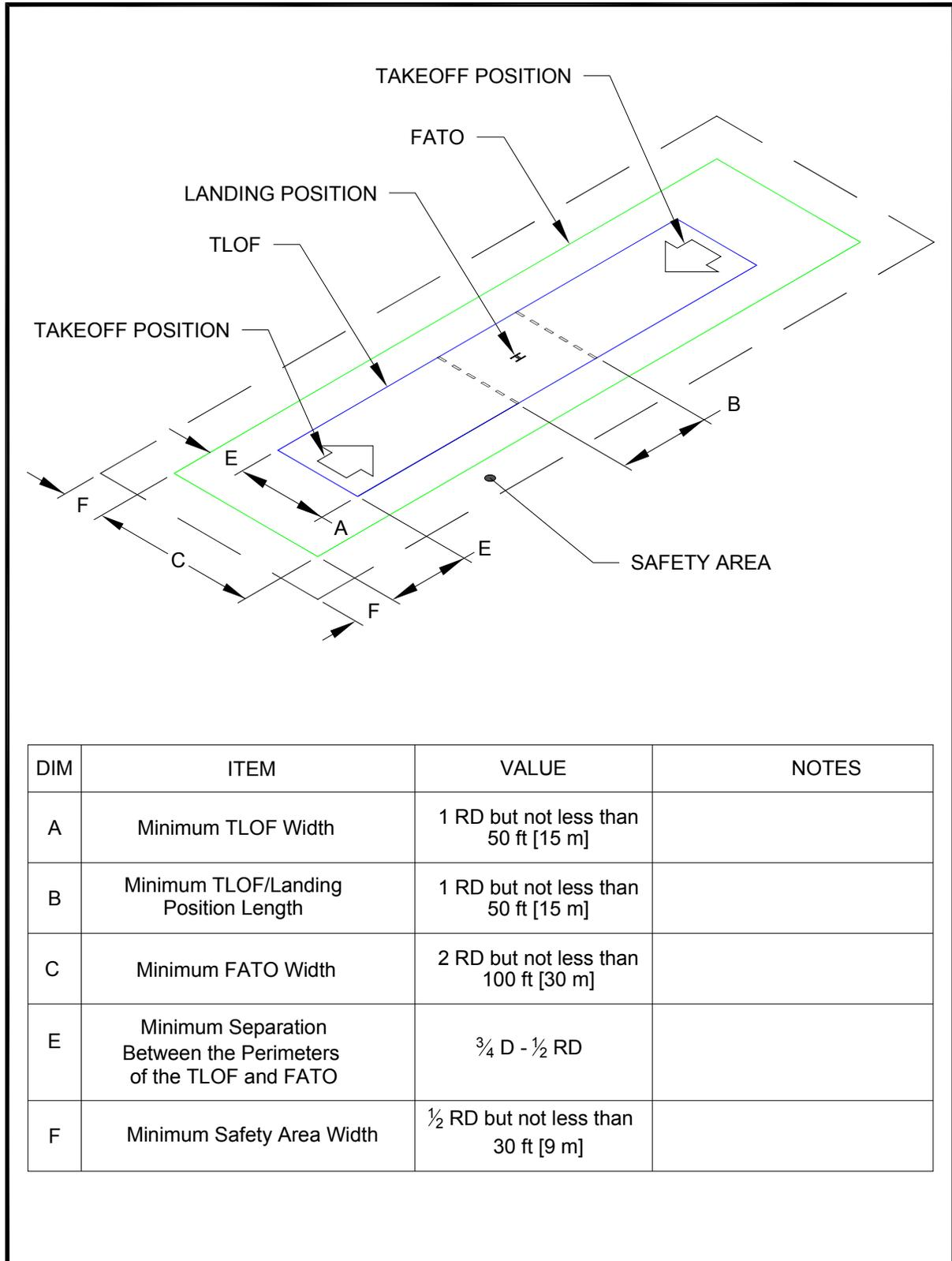
**Figure 3–3. Elongated FATO with Two Takeoff Positions: Transport**
