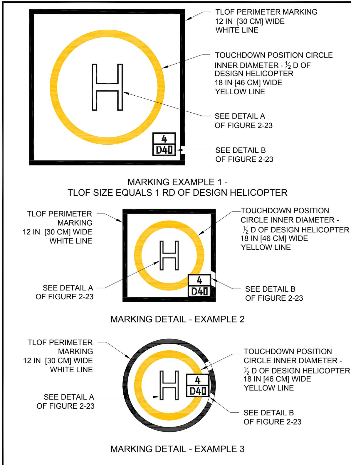
**Figure 2-22. Standard and Alternate TLOF Marking:
