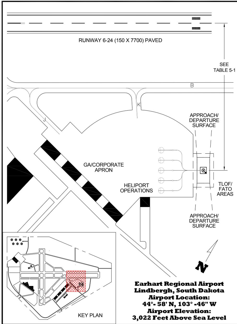
Figure 5-1. Helipont Located on an Airport: On Airport
