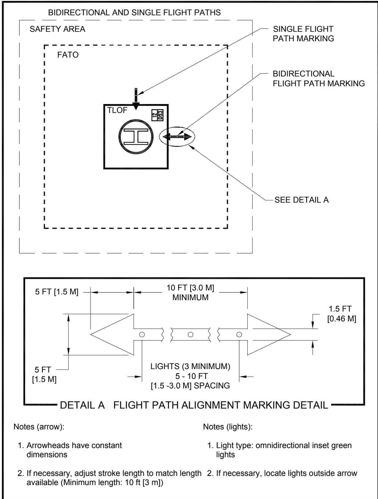
**Figure 3-9. Flight Path Alignment Marking and Lights: Transport**
