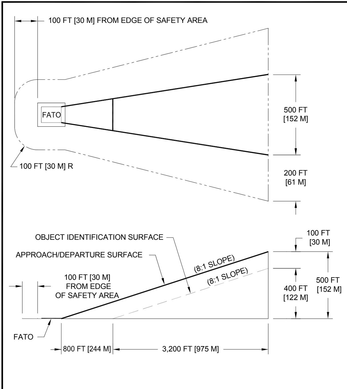
**Figure 2–32. Airspace Where Marking and Lighting are Recommended:
