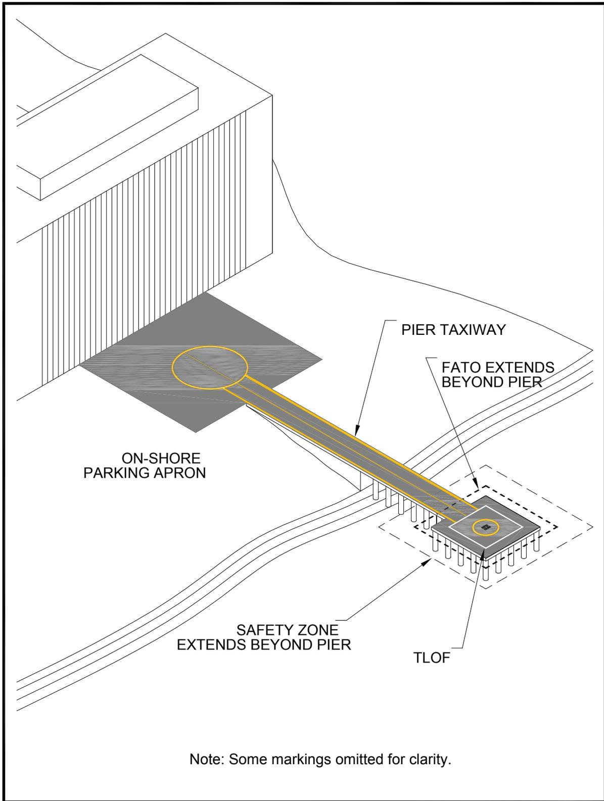
**Figure 2-6. Non-load-bearing FATO and Safety Area: General Aviation**
