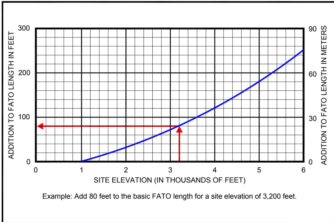
**Figure 2-5. Additional FATO Length for Helicopters at Higher Elevations:
