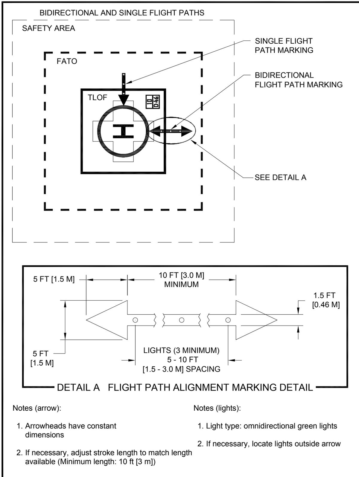
**Figure 4-10. Flight Path Alignment Marking and Lights: Hospital**
