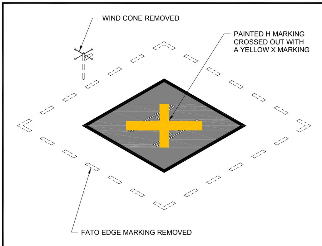
**Figure 2–27. Marking a Closed Heliport: General Aviation**
