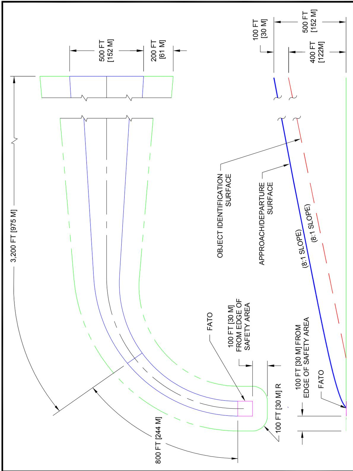
**Figure 2-33. Airspace Where Marking and Lighting are Recommended:
