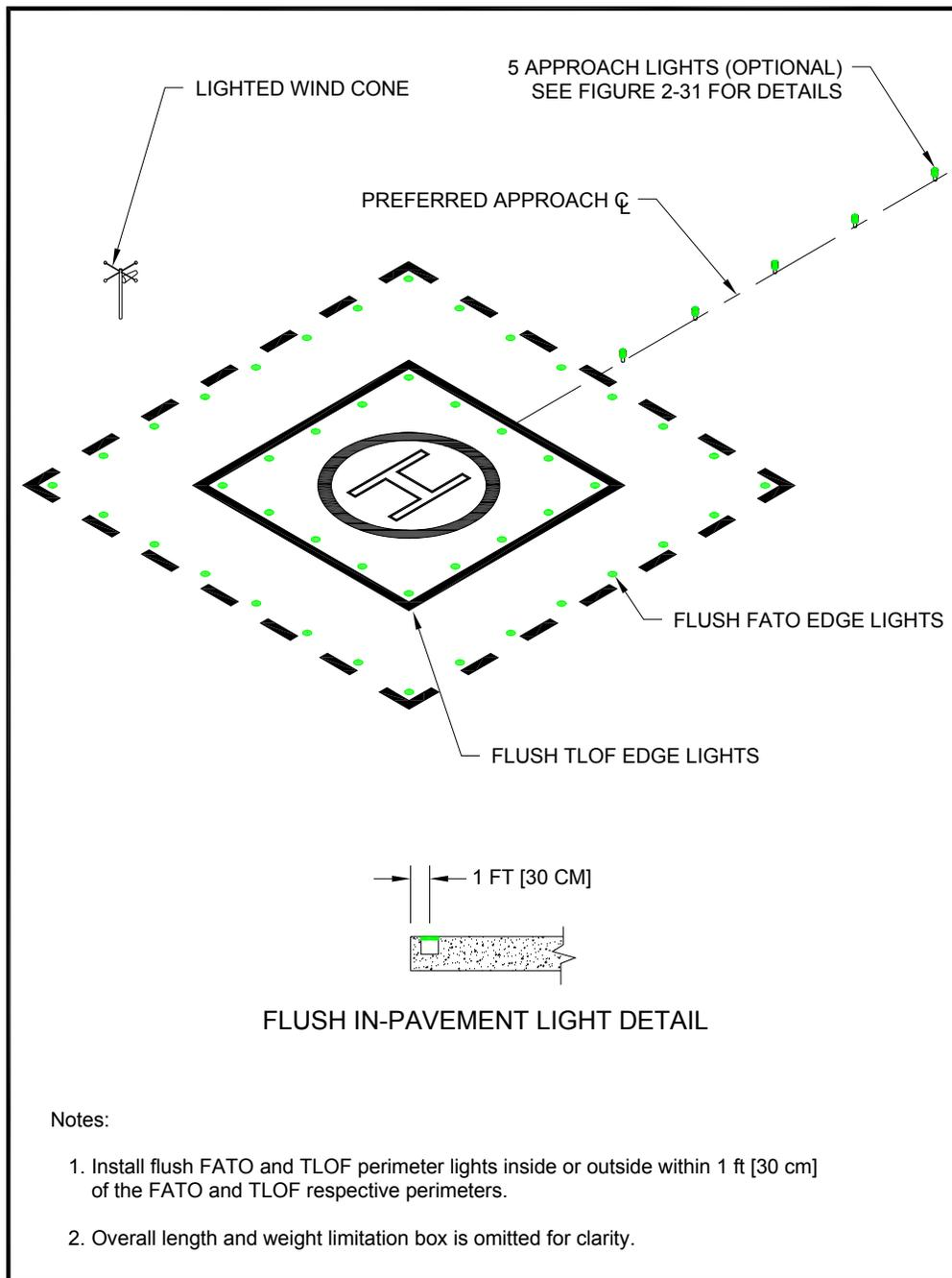
**Figure 2–29. TLOF/FATO Flush Perimeter Lighting: General Aviation**
