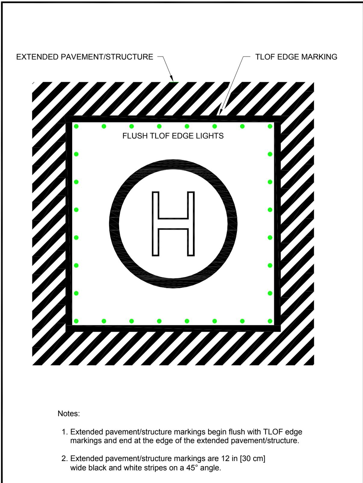
**Figure 2–24. Extended Pavement / Structure Marking: General Aviation**
