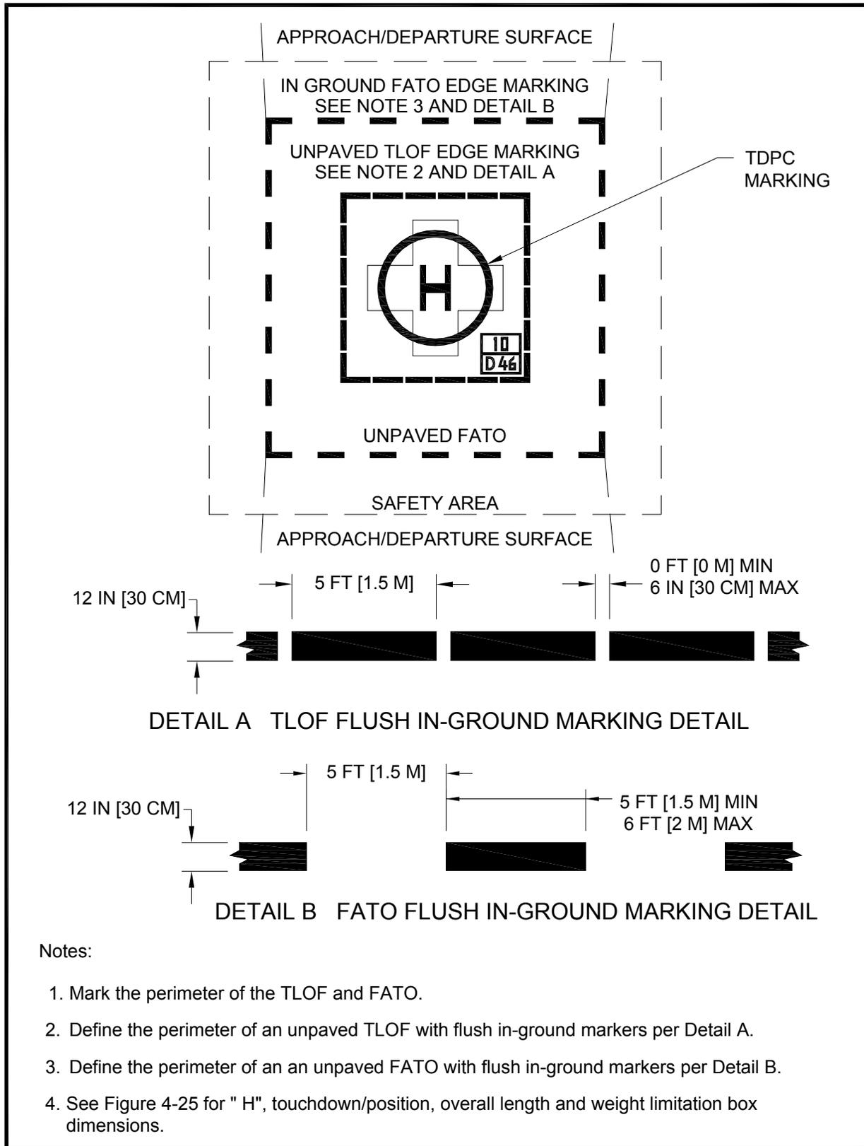
Figure 4-24. Unpaved TLOF/Unpaved FATO – Marking: Hospital
