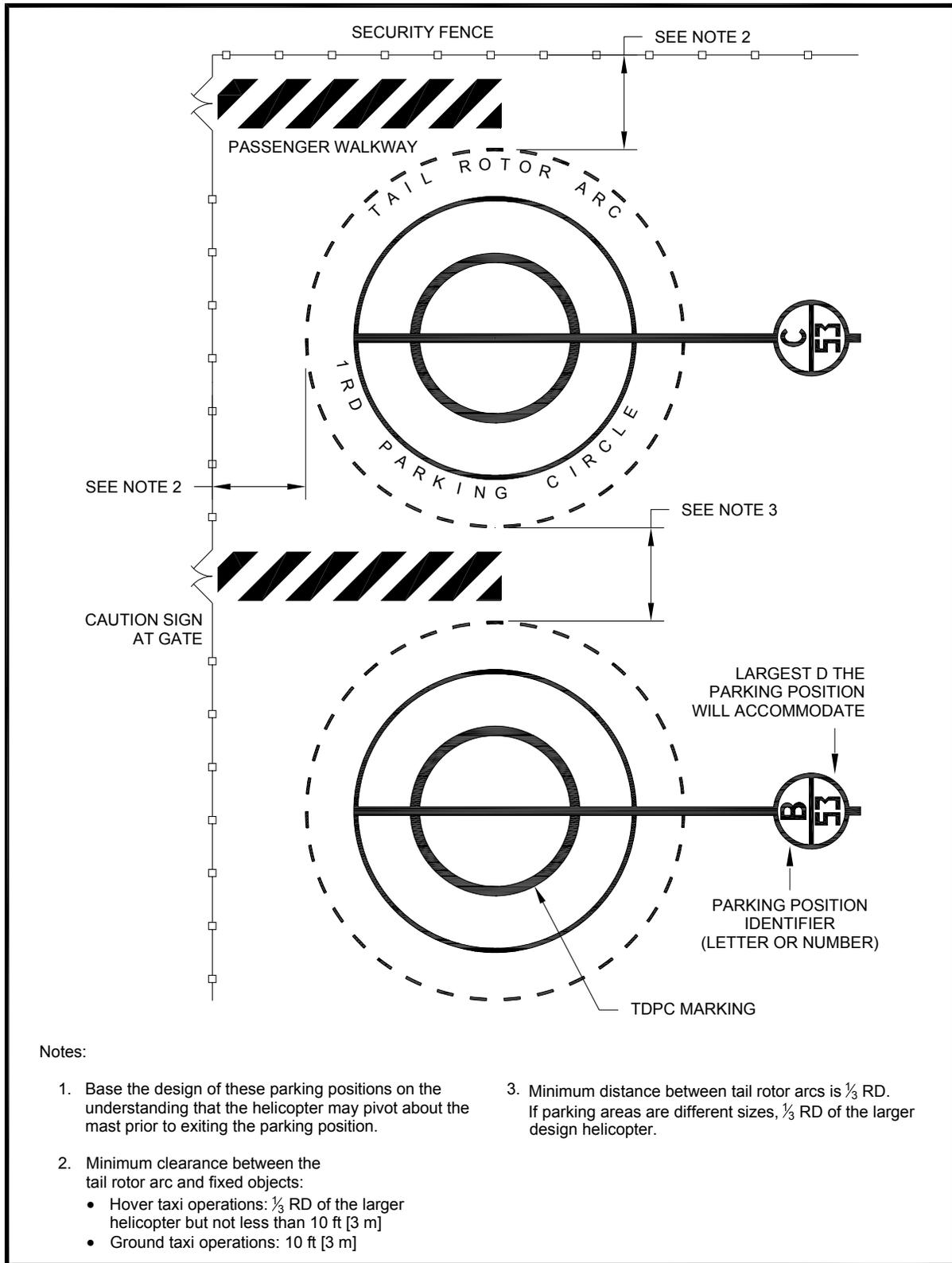
Figure 3-12. "Turn-around" Helicopter Parking Position Marking: Transport
