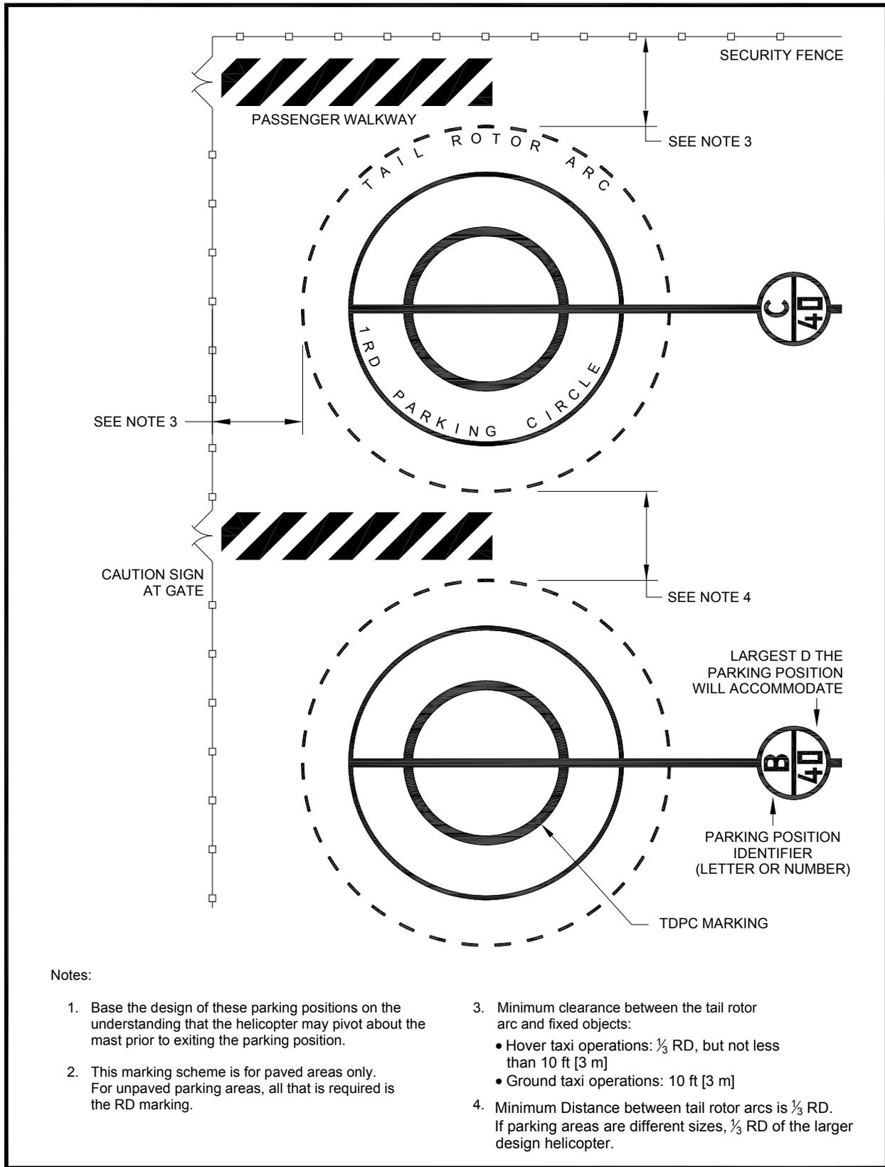
Figure 2-19. "Turn-around" Parking Position Marking: General Aviation
