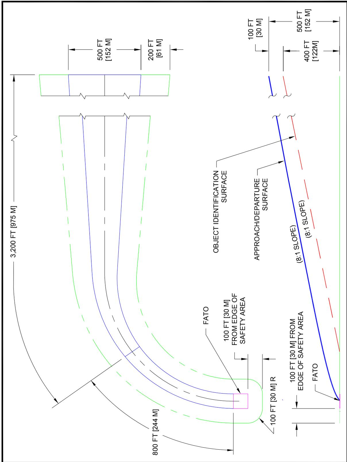
Figure 4-33. Airspace Where Marking and Lighting are Recommended:
