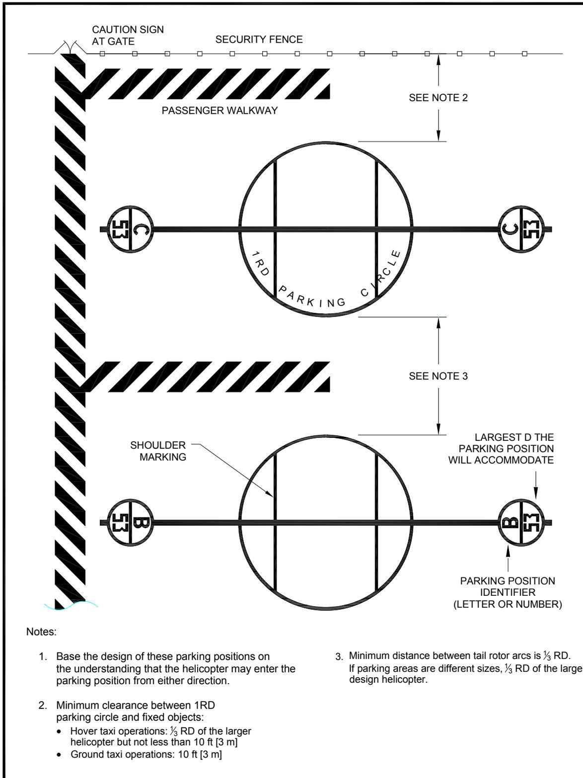
Figure 3-13. “Taxi-through” Helicopter Parking Position Marking: Transport
