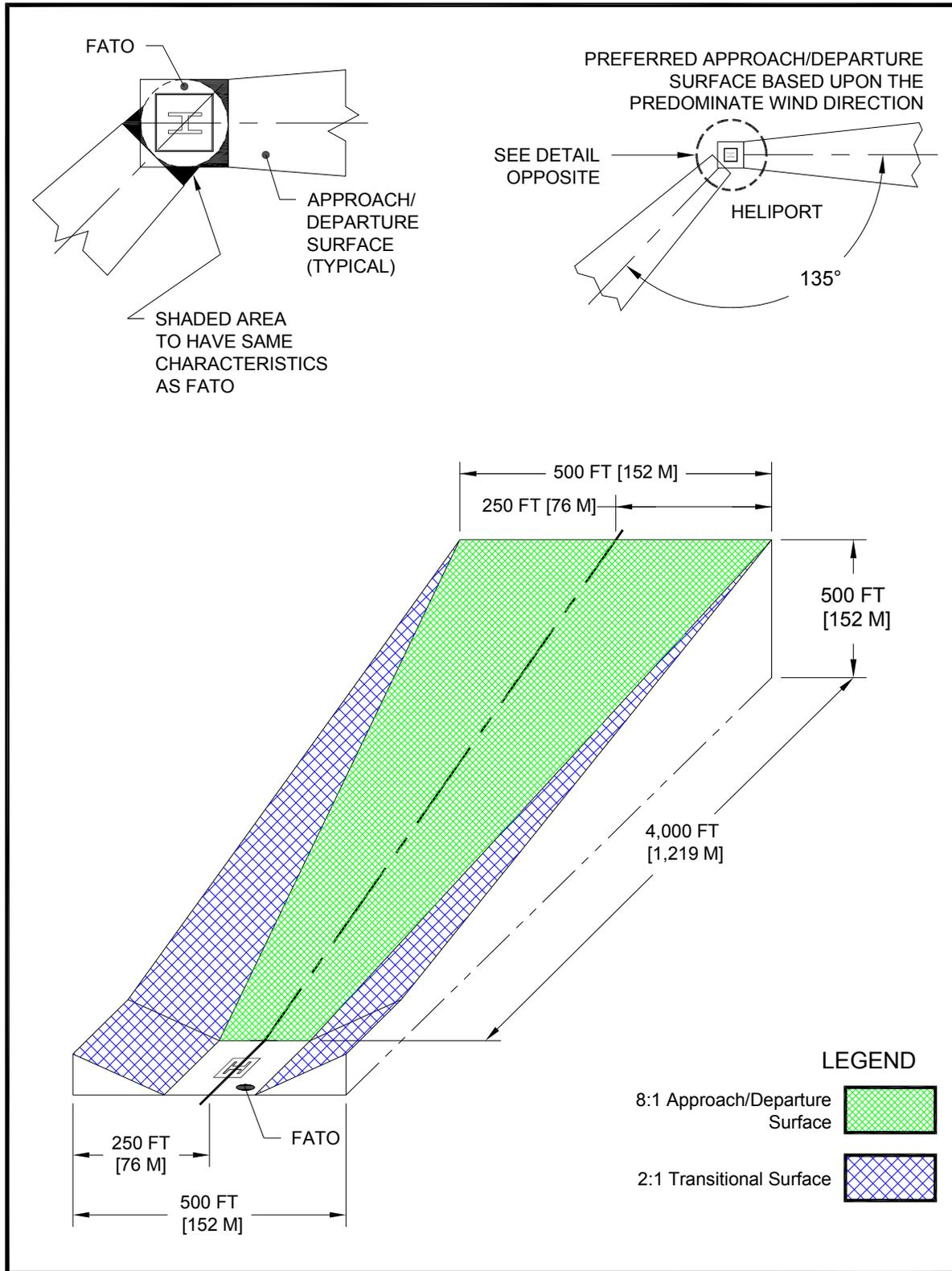
**Figure 3-7. VFR Heliport Approach/Departure and Transitional Surfaces: Transport**
