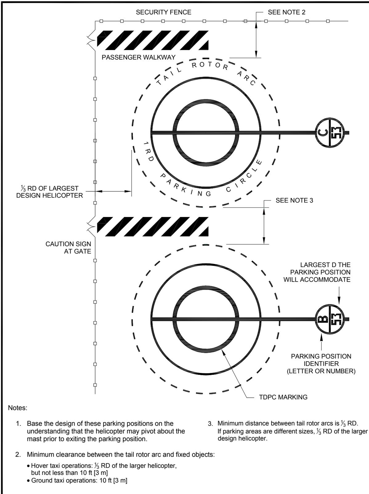
Figure 4-18. "Turn-around" Helicopter Parking Position Marking: Hospital
