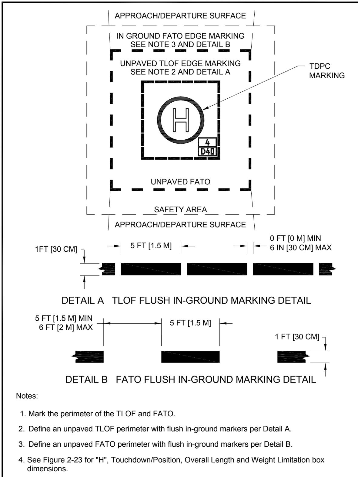
**Figure 2-26. Unpaved TLOF/Unpaved FATO – Marking: General Aviation**
