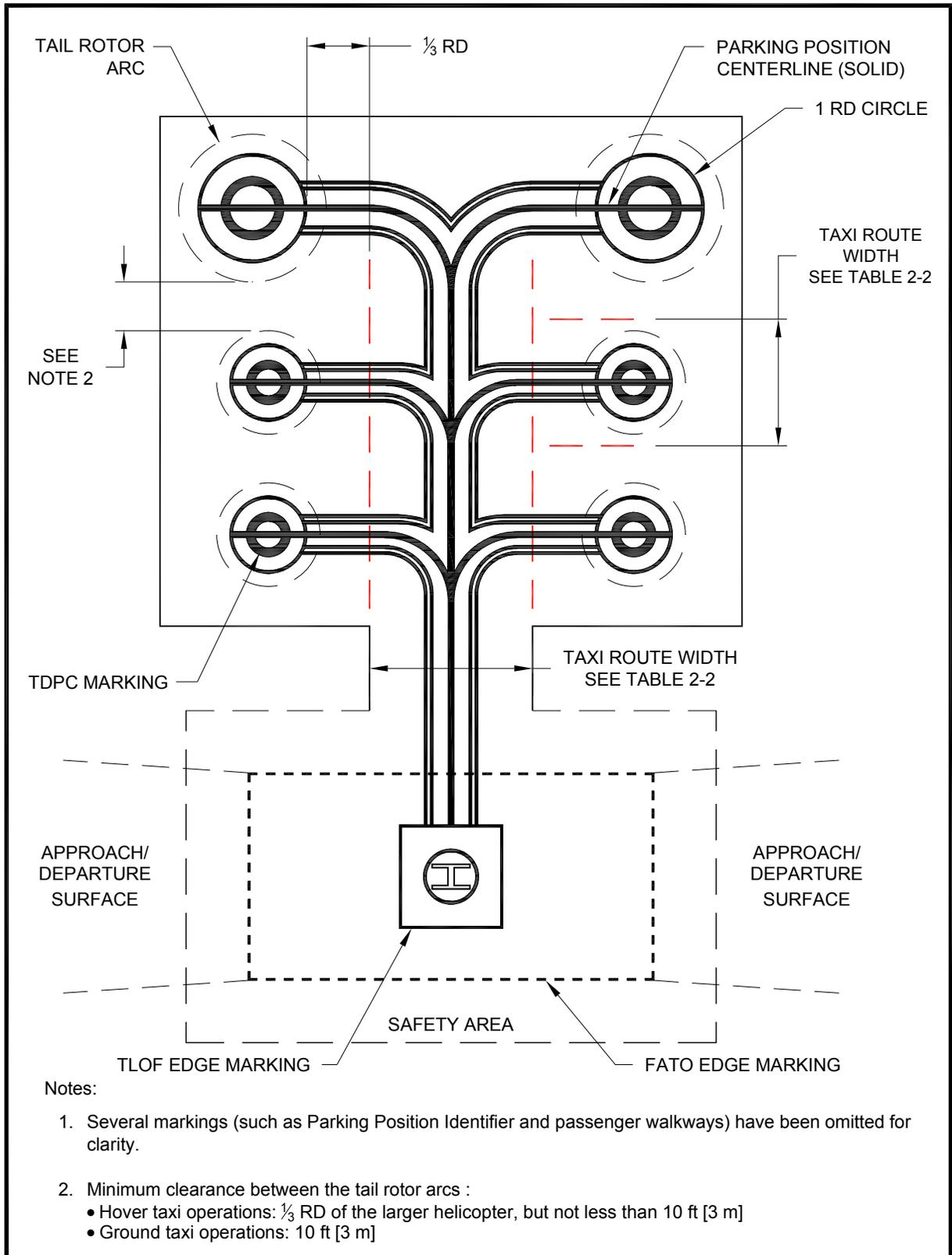
**Figure 3-14. Parking Area Design – “Turn-around” Parking Positions: Transport**
