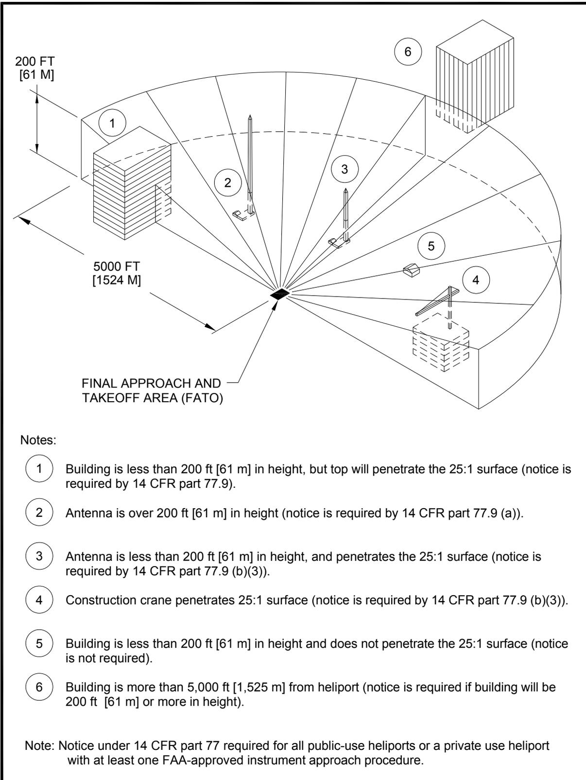
**Figure 1-4. Offsite Development Requiring Notice to the FAA**
