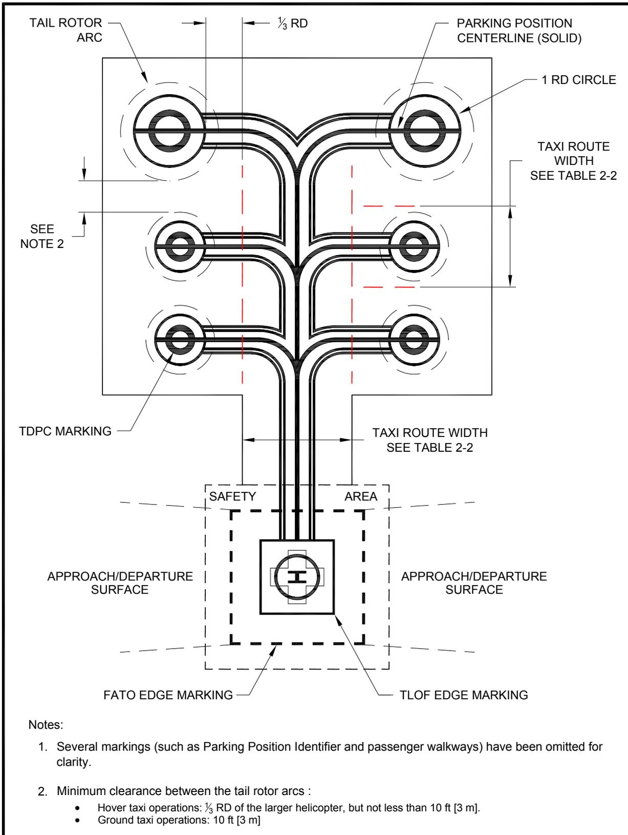
**Figure 4–16. Parking Area Design – “Turn-around” Parking Positions: Hospital**
